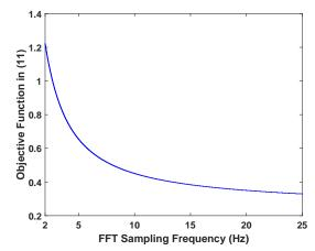
Figure 5. Residual error in state estimation obtained from objective function in (11) for different FFT sampling frequencies.
