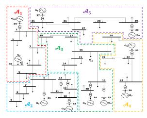
Figure 8. The IEEE 39 bus test system is partitioned into five areas.
