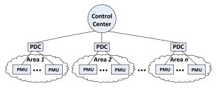
Figure 7. The hierarchical structure of a typical synchrophasor network.
